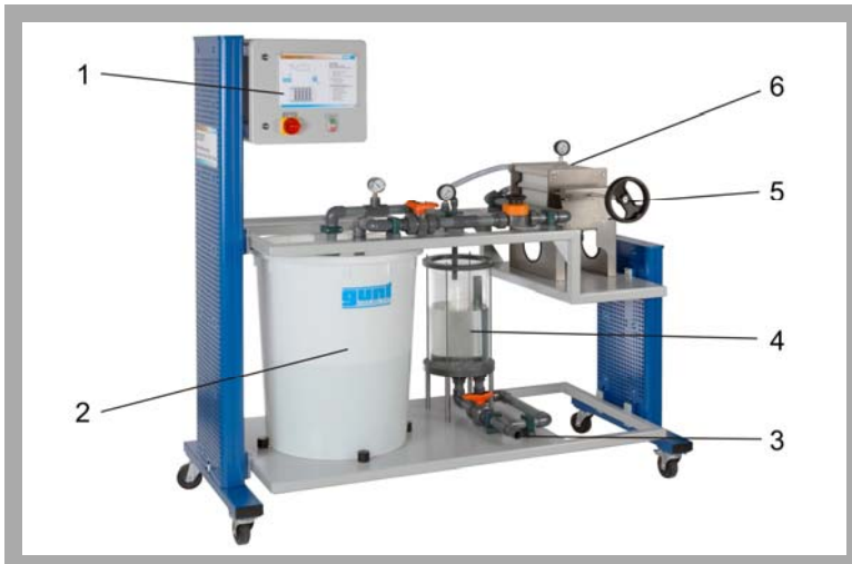
1 switch cabinet with controls, 2 suspension tank, 3 filtrate tank outlet and overflow, 4 filtrate tank, 5 spindle, 6 plate and frame filter press
